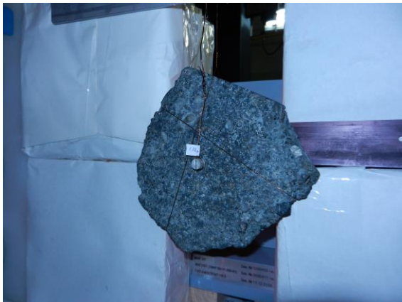
Fig. 2. Diamond simulant weighing 1.78 g behind a kimberlite sample.
