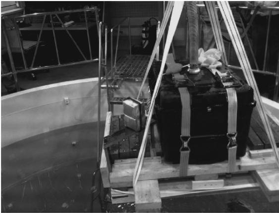
**Fig. 6.** Installation of the inspected melamine sample on the test bench.
