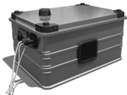
**Fig. 4.** Inspection module of a portable DVIN-1 system for the detection of explosives [10].
