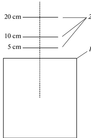
Fig. 1. Scheme of modeled conditions used in the calculation of fast-neutron flux absorption in the water medium. The estimation planes 2 are located at 5, 10, and 20 cm apart from the container housing *I*. The dashed line shows the symmetry axis of the central tagged beam.
