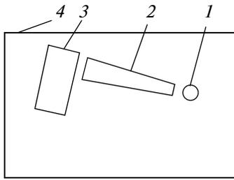
**Fig. 2.** Setup diagram: (1) fast-neutron generator, (2) protection of gamma detectors, (3) gamma-ray detectors, and (4) the detector housing.
