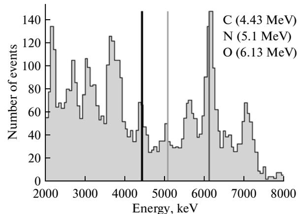
**Fig. 10.** Energy spectrum of melamine located 20 cm from the inspection module wall in water. The straight lines indicate the complete energy absorption peaks of the characteristic gamma radiation from carbon  $E_\gamma = 4.43$  MeV, nitrogen  $E_\gamma = 5.1$  MeV, and oxygen  $E_\gamma = 6.13$  MeV.
