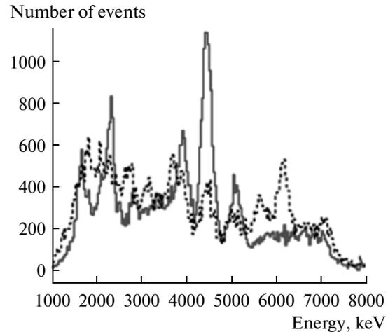
**Fig. 3.** Spectra of gamma radiation due to the irradiation of a melamine sample by fast neutrons when the sample is placed in water (dashed line) and in air (solid line).
