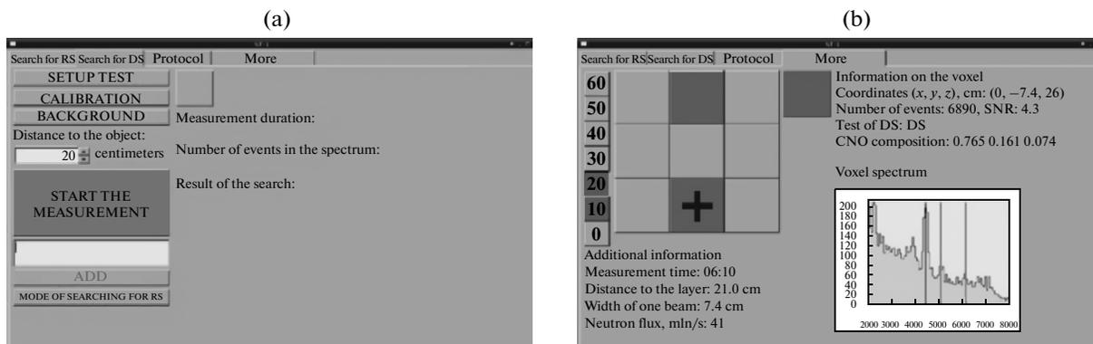
**Fig. 7.** Outward appearance of the software for analyzing the data from the DVIN-1 system: (a) operation in the mode of searching for explosives; (b) operation in the mode of analyzing the measurement results.
