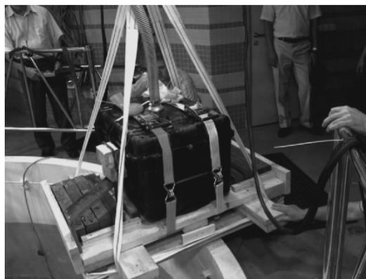
**Fig. 5.** Test bench based on a portable DVIN-1 detector for the detection of explosives.
