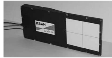
Fig. 5. The profilometer used to measure spatial distributions of the neutron tagged beams. The working area is marked by the white sheet with the cross.
