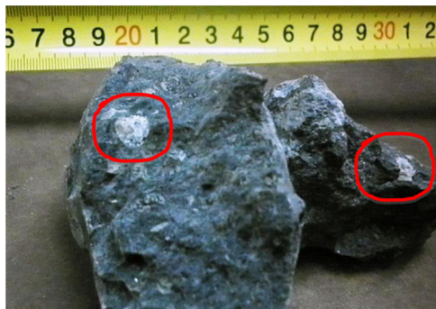
Fig. 8. Two diamond inclusions found in kimberlite sample No. 17.
